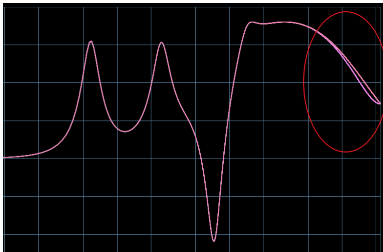
Figure 10: The difference on spectrum between minimum-phase and analogue prototype.
